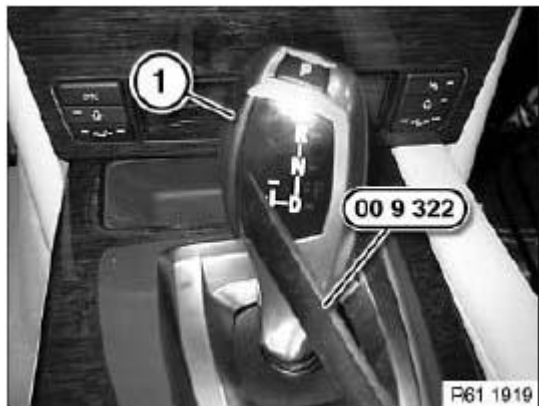
Fig. 252: Identifying Special Tool (00 9 322)
