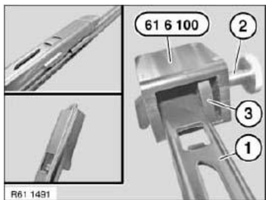
Fig. 336: Inserting Windscreen Wiper Arm In Special Tool (61 6 100)
