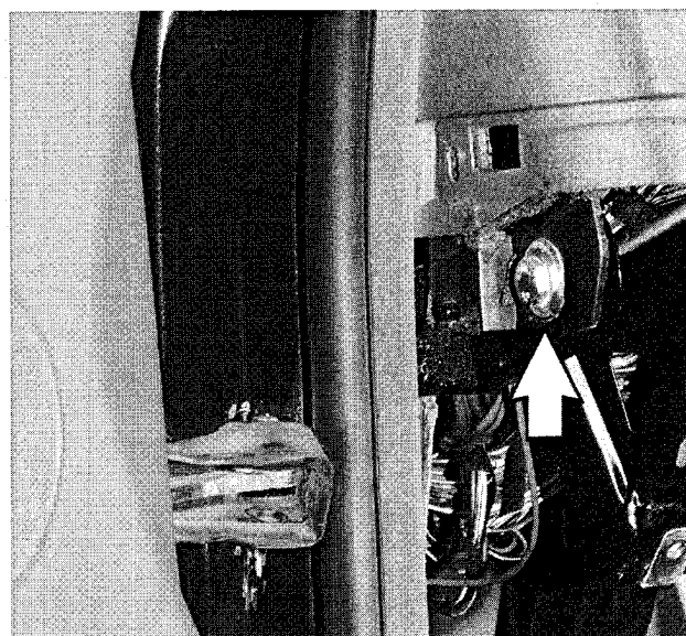
Fig. 10. Dashboard mounting bolt (arrows). Left side shown, right is similar. Some models may have two bolts on each side.
