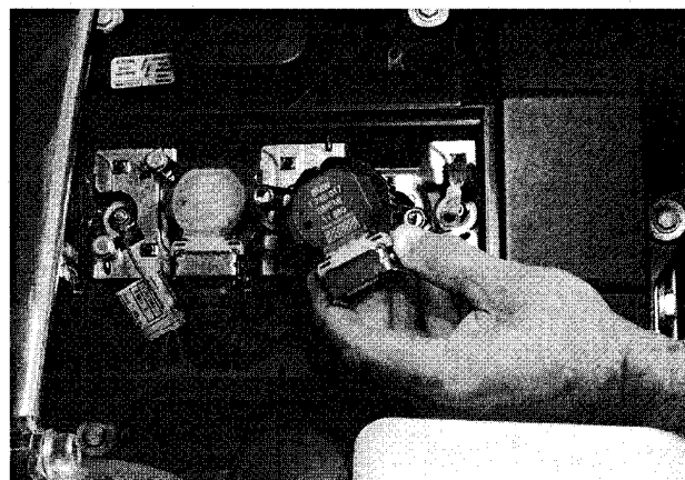
Fig. 17. Six-cylinder ignition coil in top of cylinder head (M52 engine).
