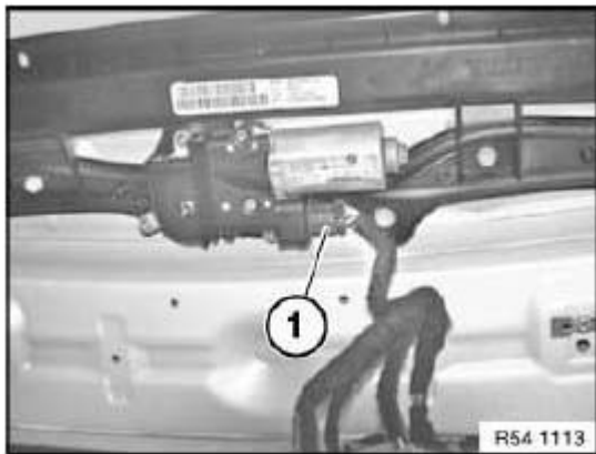
Fig. 55: Identifying Plug Connection
