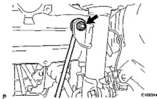
Fig. 49: Locating Nut And Stabilizer Link Courtesy of TOYOTA MOTOR SALES, U.S.A., INC.
