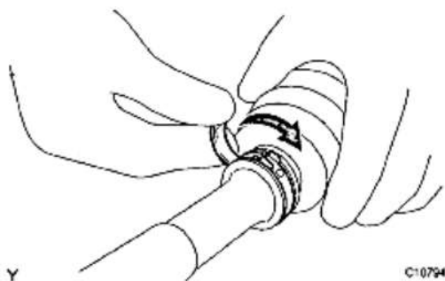
Fig. 37: Installing Boot Clamp Onto Inboard Joint Boot Courtesy of TOYOTA MOTOR SALES, U.S.A., INC.
