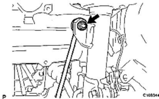
Fig. 6: Locating Nut And Stabilizer Link Courtesy of TOYOTA MOTOR SALES, U.S.A., INC.
