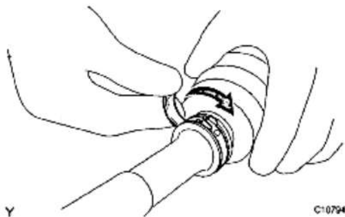
Fig. 28: Installing Boot Clamp Onto Outboard Joint Boot Courtesy of TOYOTA MOTOR SALES, U.S.A., INC.
