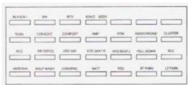
Cadillac Eldorado – fuse box diagram – trunk
