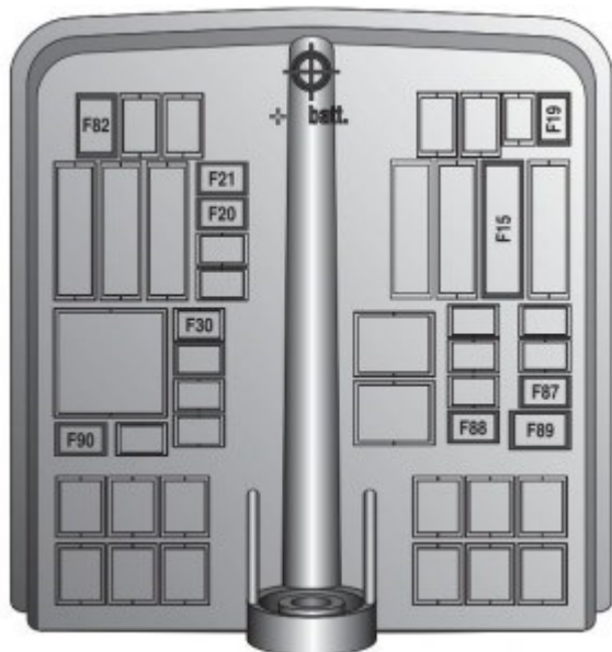
Fiat Panda mk3 – fuse box- engine compartment
