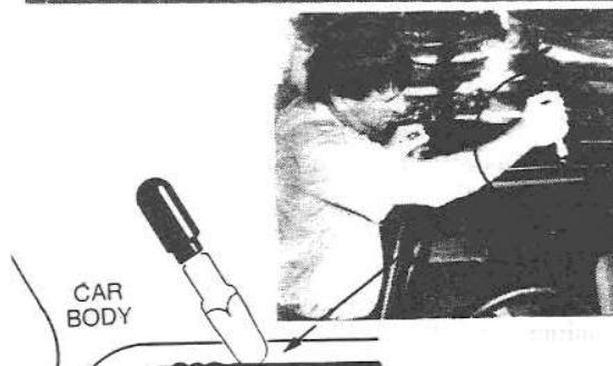
Trim excess sealant from the external edge of the windscreen
