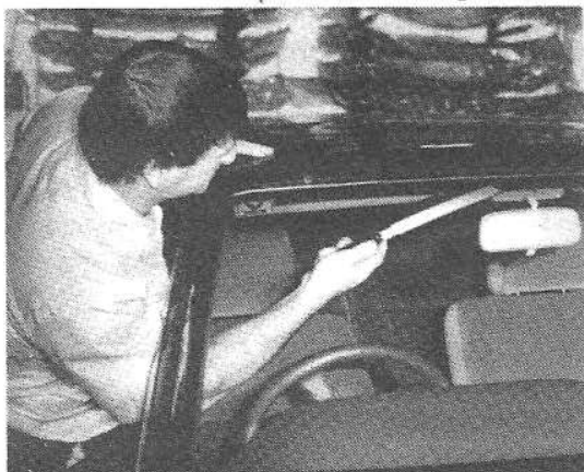
BTB Windscreen removal tools. Using a manual handle blade
