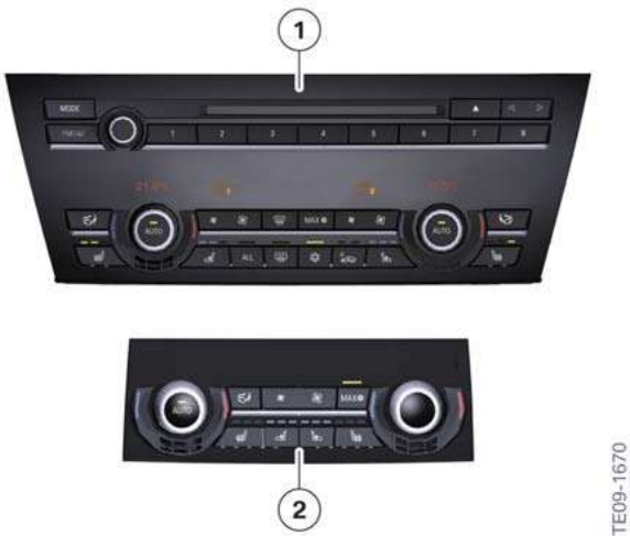
F10 Control panels for the 4-zone IHKA
