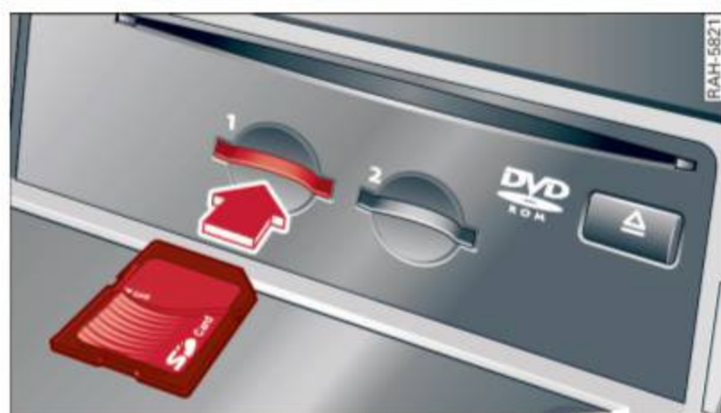
Fig. 6 Inserting a memory card
