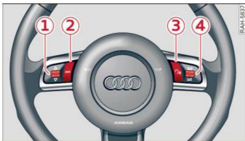
Fig. 72 Controls on the multifunction steering wheel
