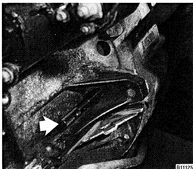
Fig. 23. BMW special tool no. 11 2 300 installed through bellhousing and into flywheel.
