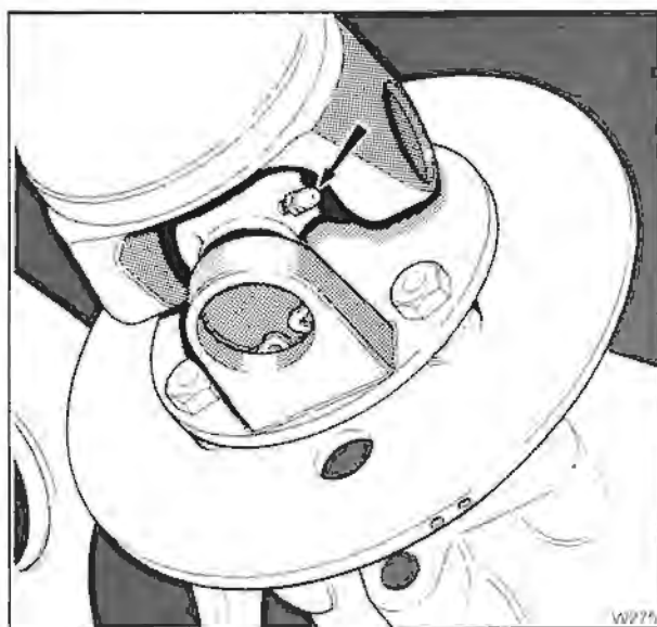
Fig. B2-26 Propeller shaft grease point
