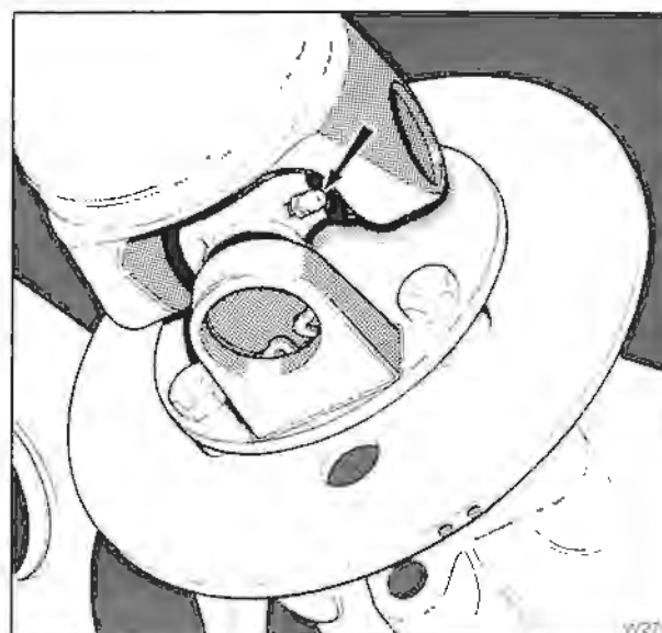
Fig. B1-22 Propeller-shaft grease point
