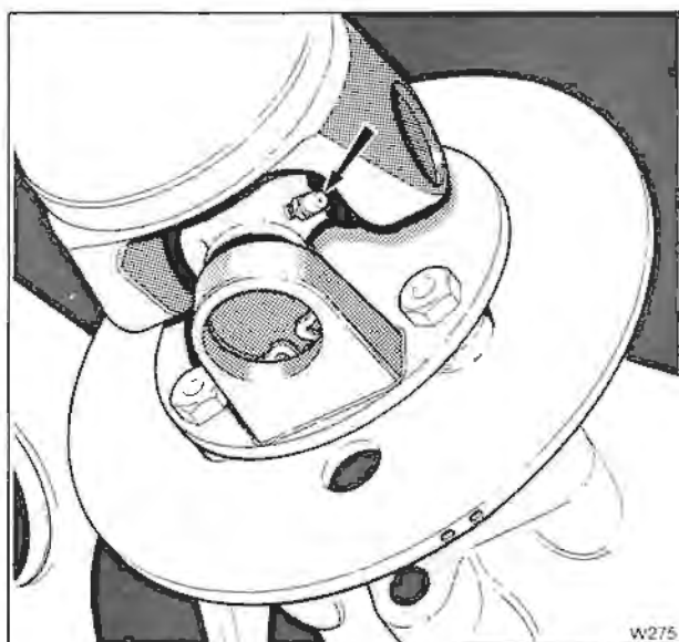
Fig. B1/1-17 Propeller-shaft grease point
