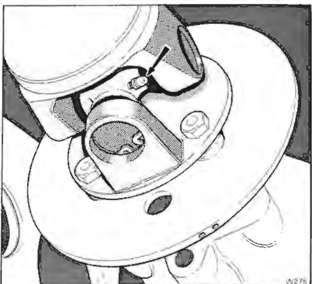
Fig. B4-31 Propeller shaft grease point
