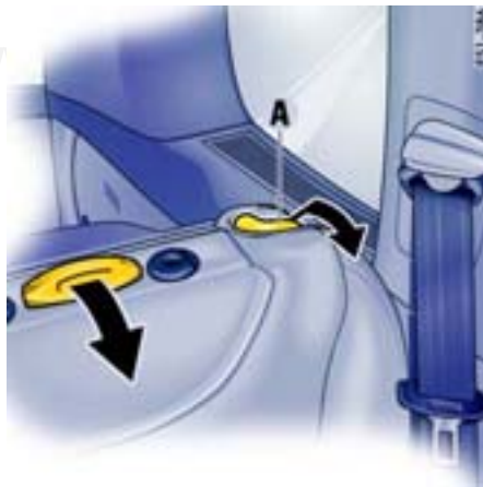
6. Pull release lever A and fold the backrest forward.
