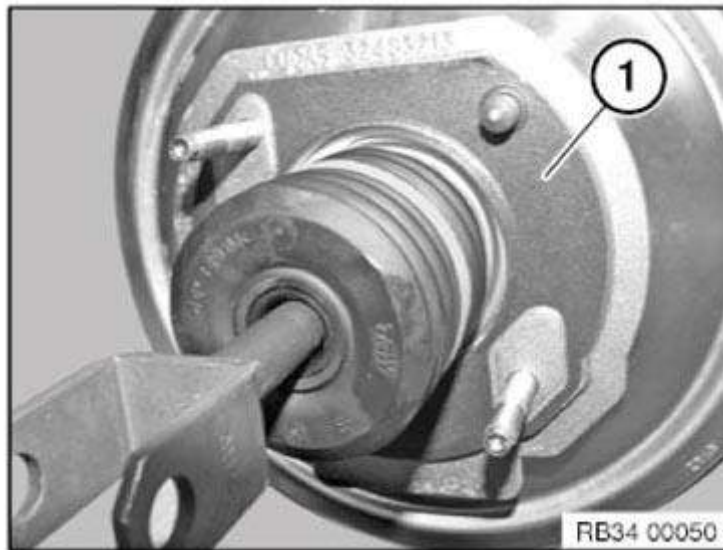
Fig. 172: Identifying Protective Film On Connection Of Vacuum Line
