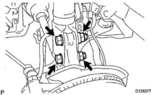
Fig. 60: Locating Nuts And Bolts Courtesy of TOYOTA MOTOR SALES, U.S.A., INC.
