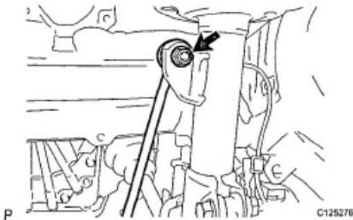
Fig. 62: Locating Nut And Stabilizer Link Courtesy of TOYOTA MOTOR SALES, U.S.A., INC.
