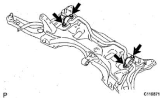
Fig. 84: Locating Bolts And Stabilizer Bracket Courtesy of TOYOTA MOTOR SALES, U.S.A., INC.
