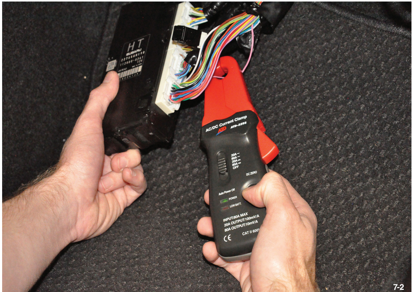
Injector Current Draw Test
