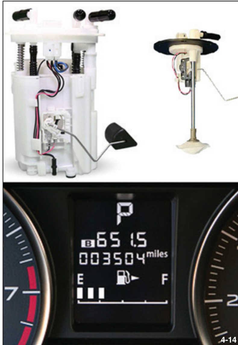
Primary and Secondary Fuel Level Sensors
