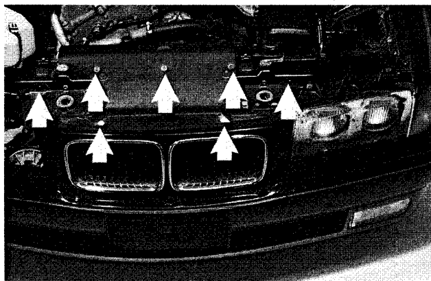
Fig. 2. Radiator cover screws (arrows).
