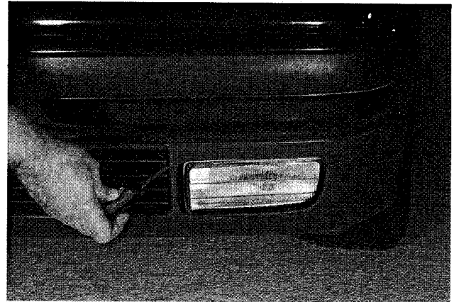
Fig. 8. Insert screwdriver in upper air duct inlet.
