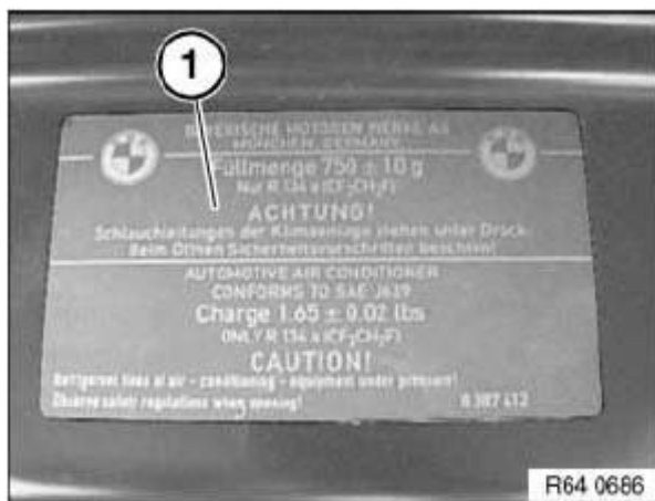
Fig. 80: Identifying A/C System Is Contained On Rating Plate Courtesy of BMW OF NORTH AMERICA, INC.
