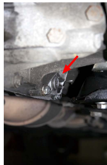
Drain plug (pictures were taken after the oil change, that's why the gearbox is dirty of oil)
