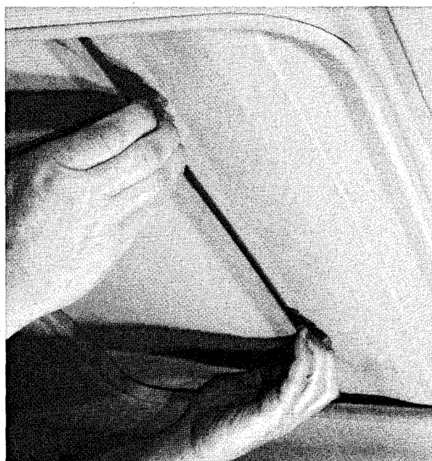
Fig. 4. Slide sunroof liner back into roof cavity.
