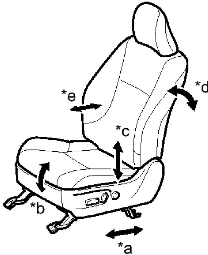
Fig. 7: Identifying Front Power Seat Function Courtesy of TOYOTA MOTOR SALES, U.S.A., INC.
