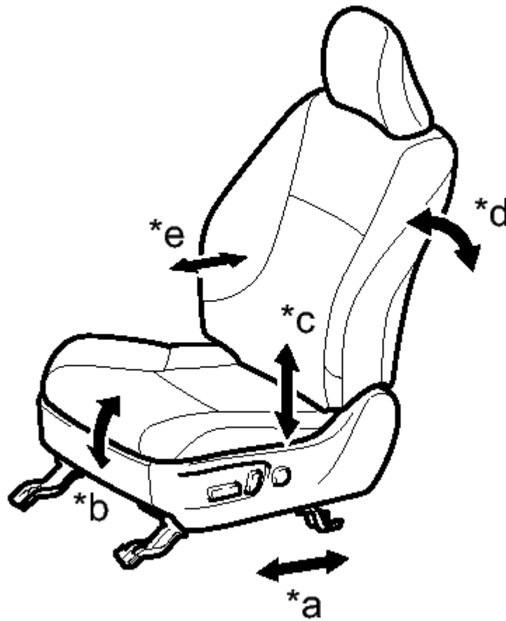
Fig. 4: Identifying Front Power Seat Function Courtesy of TOYOTA MOTOR SALES, U.S.A., INC.
