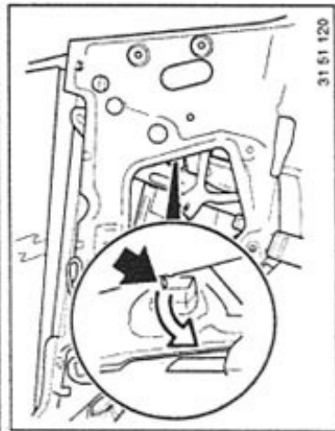
Loosen screw and push back main stop maximum distance.
