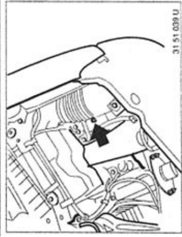
Unfasten hose clips on left and right sides of air manifold.
