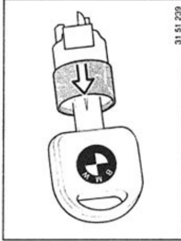
Remove metal ring. Carefully remove main key from locking cylinder. Remove metal ring and reinsert main key in the locking cylinder.
