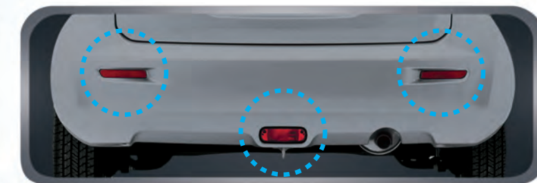
Rear Bumper with Reflector & Rear Fog Lamp
