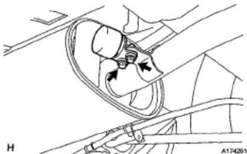
Fig. 21: Locating Bolts And Exhaust Pipe Damper Courtesy of TOYOTA MOTOR SALES, U.S.A., INC.
