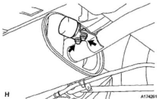
Fig. 35: Locating Bolts And Exhaust Pipe Damper Courtesy of TOYOTA MOTOR SALES, U.S.A., INC.
