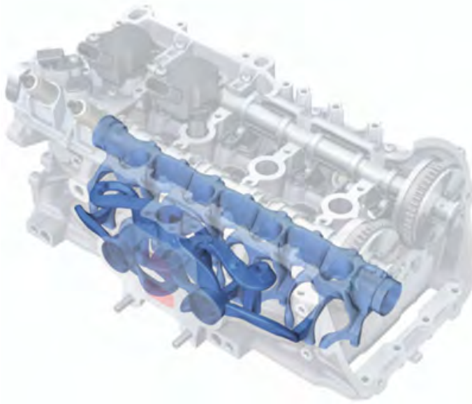
Cooling ducts of integrated exhaust manifold
