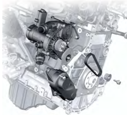
Installation position of actuating element for engine temperature control
