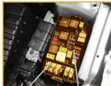
Multi-fuse pre-fuse holder SA on the relay and fuse carrier SR1
