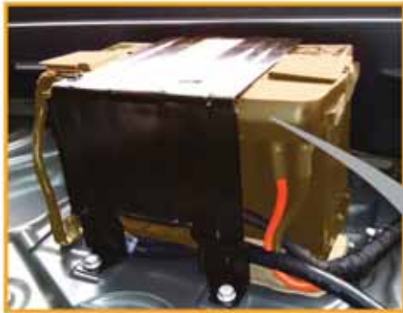
12-V battery with main fuse box central in the luggage compartment close to the lock carrier
