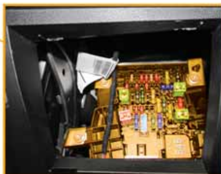
Fuse holder SC on relay and fuse carrier SR2
