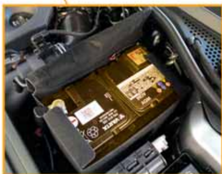
12-V battery in engine compartment
