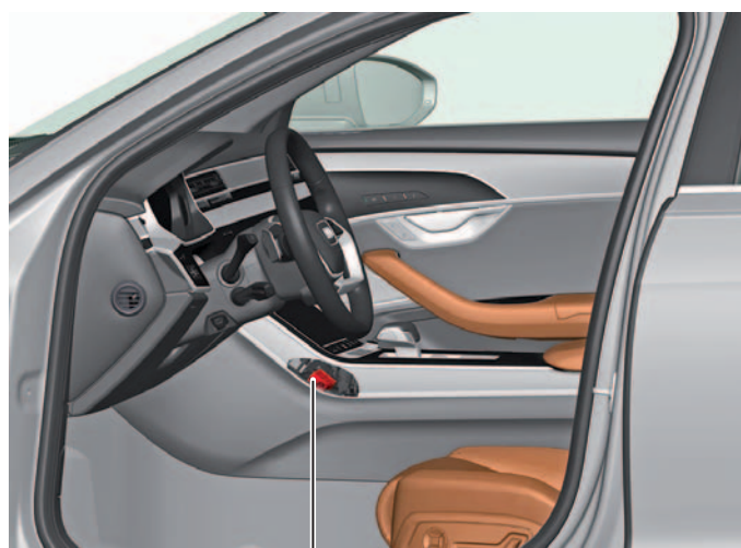
Installation position of control unit 2 for near field communication J1170
