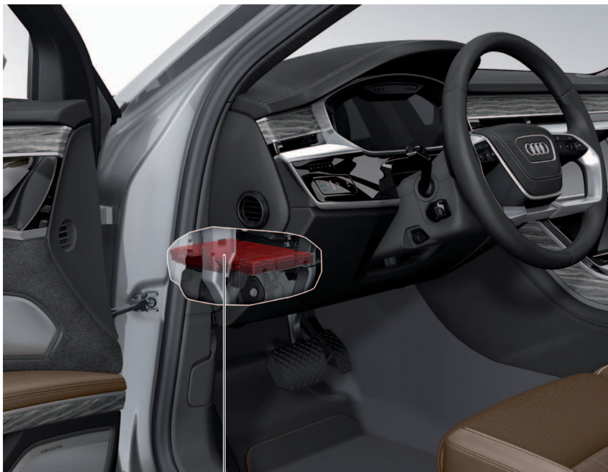
Electrical system control unit J519
