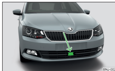
Fig. 217 Installation location of the radar sensor
