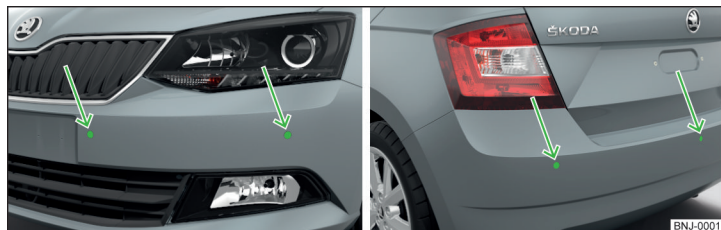
Fig. 219 Installation location of the sensors on the left side of the vehicle: front/rear
