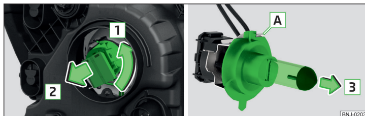
Fig. 303 Changing the bulb for the main beam
