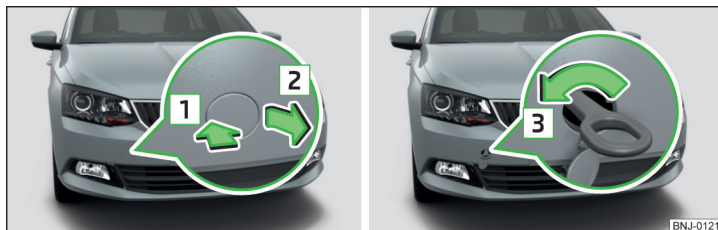
Fig. 280 Remove cap / install towing eye
