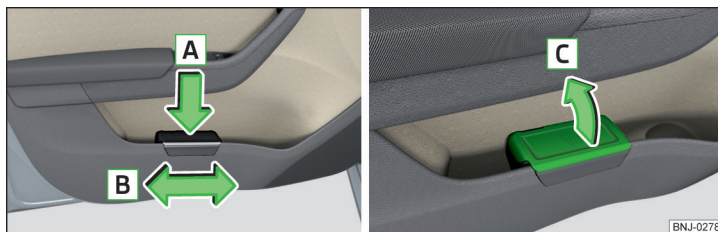
Fig. 83 Waste container: inserting and moving/opening
