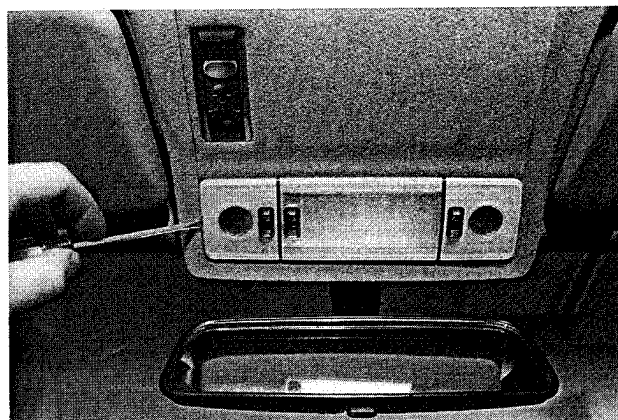
Fig. 15. Dome light assembly being removed.
