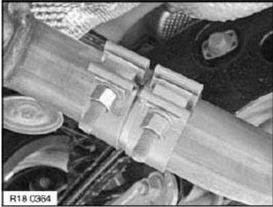
Fig. 19: Tightening Centre Clamps
