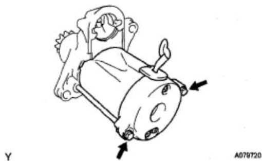
Fig. 37: Locating Starter Yoke Assembly Through-Bolts
