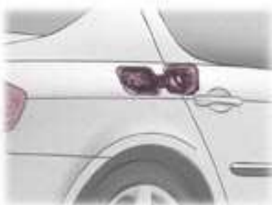
Access to the fuel filler flap
