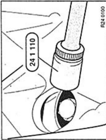
Unfasten screws and remove transmission cross-member.
