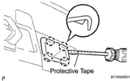
Fig. 137: Removing Protective Tape Using Screwdriver Courtesy of TOYOTA MOTOR SALES, U.S.A., INC.
