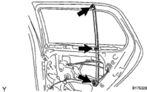
Fig. 94: Locating Bolts And Screw And Rear Door Window Division Bar Sub-Assembly Courtesy of TOYOTA MOTOR SALES, U.S.A., INC.
