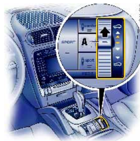
1st actuation: Terrain level
