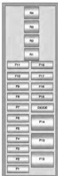
Chevrolet Volt – fuse box – instrument panel (left side)
