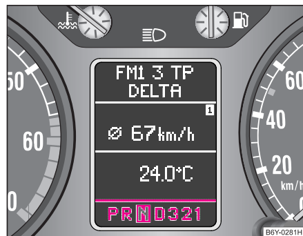
Fig. 96 Information display in the instrument cluster Selector lever positions
