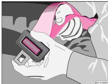
Fig. 107 Extending the pelvic belt
