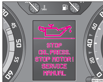
Fig. 14 Information display: Oil pressure is low
