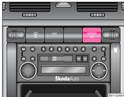
Fig. 116 Indicator light for a switched off front seat passenger airbag
