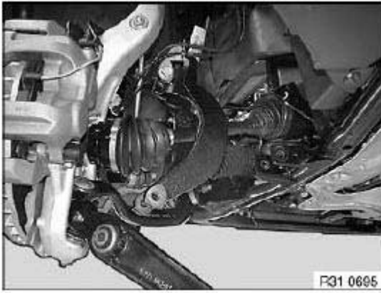
Fig. 145: Removing Output Shaft From Wheel Bearing Courtesy of BMW OF NORTH AMERICA, INC.
