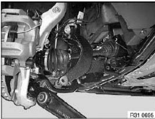
Fig. 142: Removing Output Shaft From Wheel Bearing
