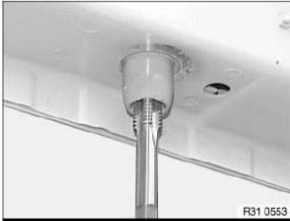
Fig. 9: Creating Locating Thread For Heli-coil Courtesy of BMW OF NORTH AMERICA, INC.
