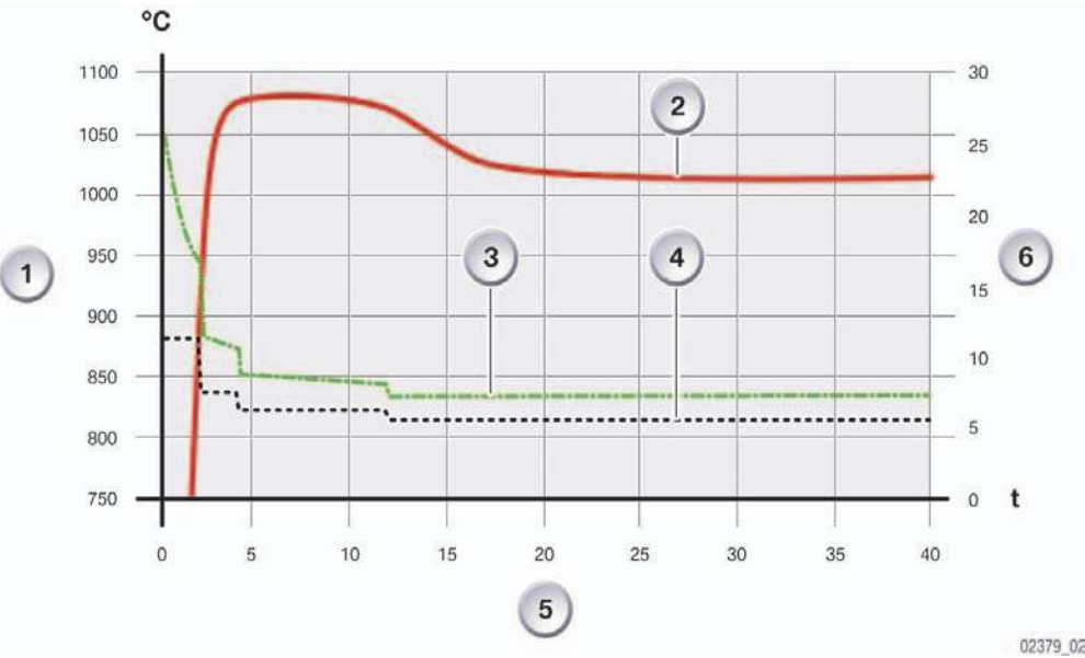
Fig. 33: Activation profile and temperature progression of glow plugs
