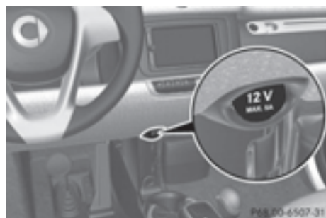
Auxiliary power outlet
