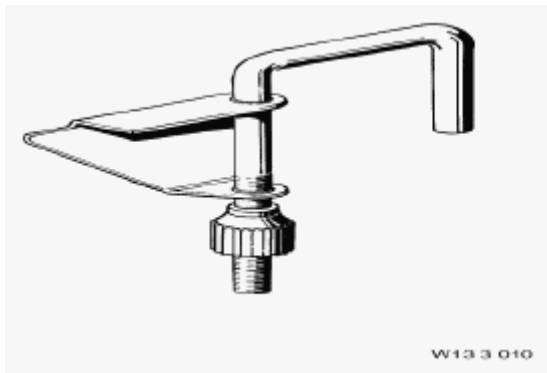
Fig. 7: Identify Special Tool (13 3 010) Courtesy of BMW OF NORTH AMERICA, INC.
