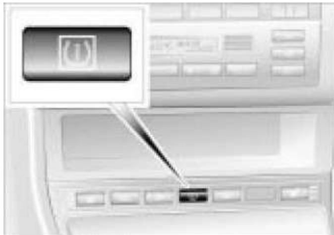
Fig. 10: Locating TPM System Reset Button (3-Series & X5 - Typical) Courtesy of BMW OF NORTH AMERICA, INC.
