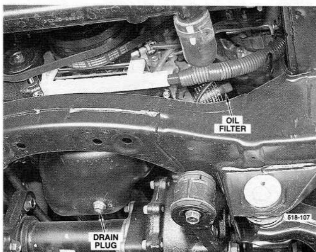
Engine sump drain plug and oil filter location. Stoneguard removed.
