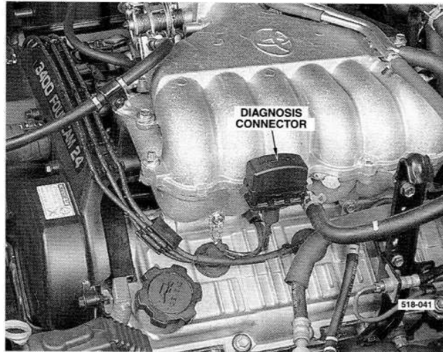
Diagnosis connector location. The terminal identification is printed on the inside of the cover.
