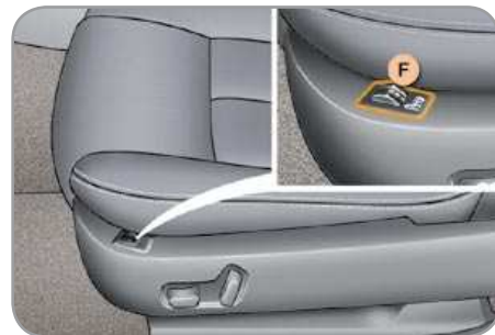
F. Heated seat adjustment.
