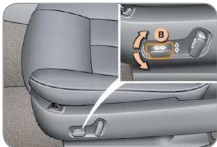
B. Seat cushion angle adjustment.
