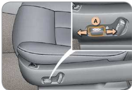
A. Forwards-backwards adjustment.
