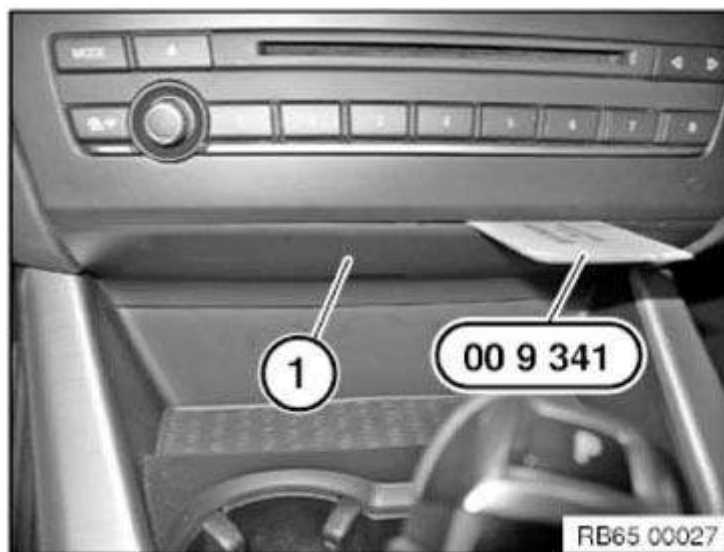
Fig. 9: Removing Trim Cover Using Special Tool 00 9 340
