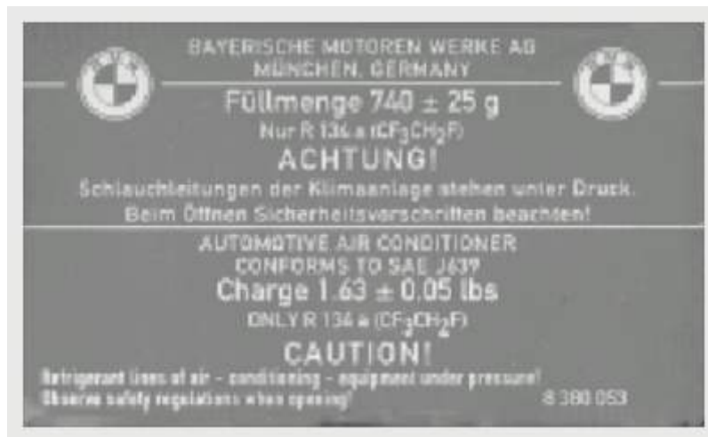
Fig. 1: Identifying Oil Used In R-134A-Charged Systems Label
