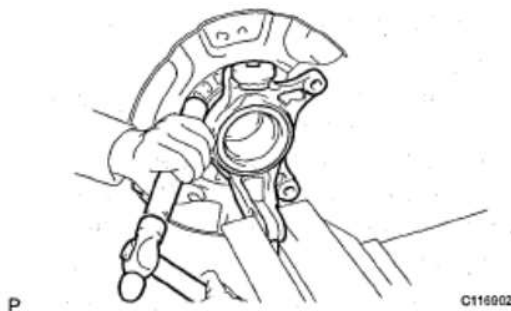
Fig. 13: Removing Dust Cover By Tapping
