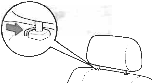
Head rest Adjustment (optional) Push button and pull/push to adjust headrest.
