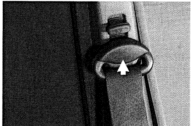
Fig. 28. B-pillar seat belt anchor trim (arrow).
