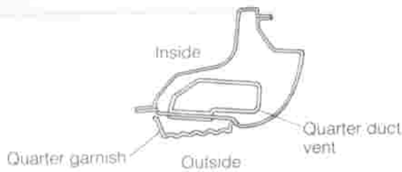
Ventilation of rear pillar section (A-A sectional view)
