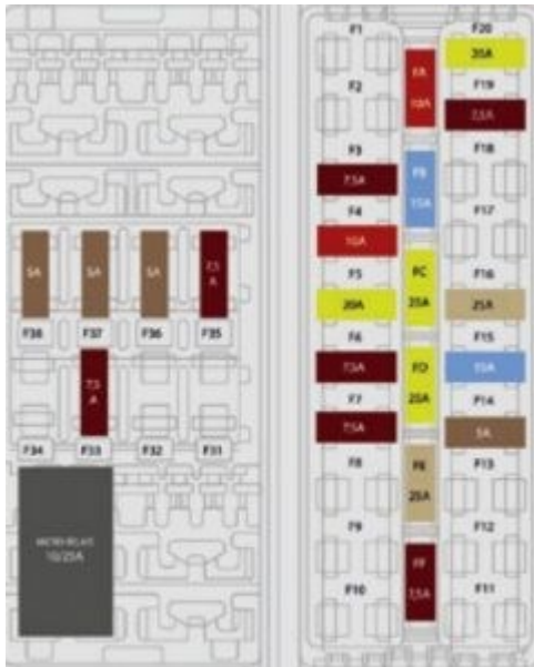
Citroen E-Mehari – fuse box diagram – passenger compartment
